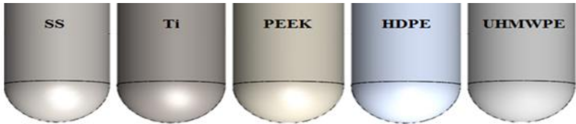
Figure 4-2 Implant models, in order of descending Young's Modulus.
