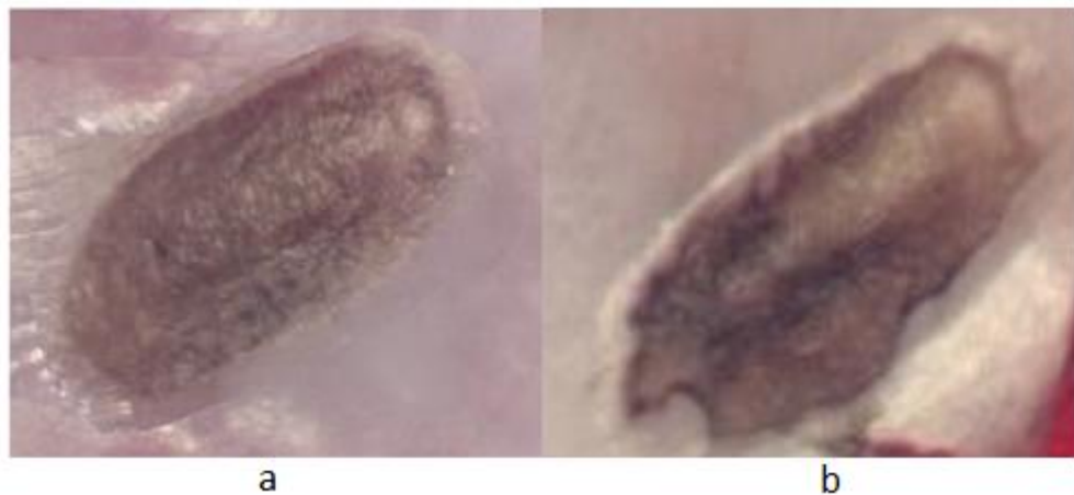
Figure 3-3 Comparison of India ink stains: a) Cartilage worn with a stainless steel pin, which shows uniform damage. b) Cartilage worn with a PEEK pin, which shows denser ink pigmentation and increased fibrillation, indicating more severe damage.
